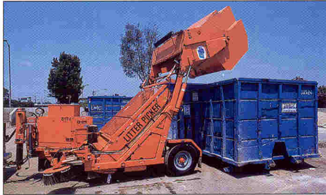
Left: Barber LP200 Litter Picker safely deposits highway litter in its four-cu yd hopper until dumping. Right: With a dump height of eight ft, the Litter Picker can empty its load into a dump truck or a roadside dumpster.
