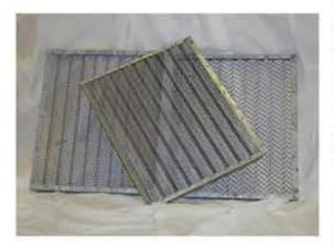
Each machine includes three (3) interchangeable screens with varying mesh sizes of 3/16" (5 mm), 3/8" (8 mm), and 1/2" (12 mm). The smaller mesh is used for ultra fine cleaning and the large mesh allows for faster and deeper cleaning, particularly in wet sand. Additional sifting screen sizes are also available.
