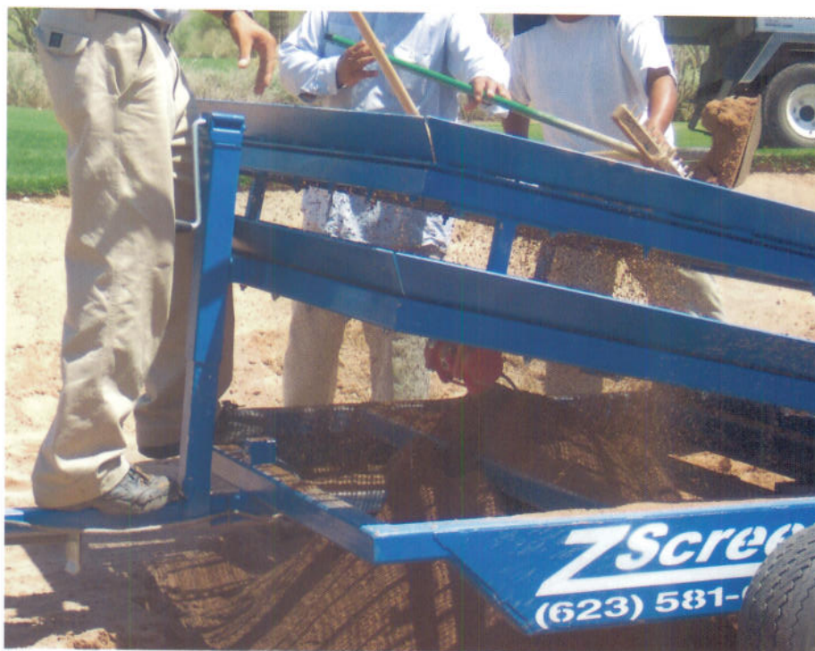
The Sand Storm from Z Screen is a double-decker vibrating screen unit.
