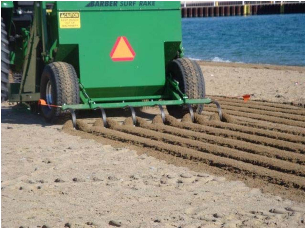
It functions by first allowing the beach cleaning machine to clean 6" deep to remove surface litter, like normal. Then the 'Chicago Rake' aerates the sand and increases the surface area exposed to the sun. With frequent cleaning, this increased sun/air exposure helps get the beaches' bacteria levels back to normal levels. In the case of Chicago's problem, the Chicago rake proved effective, and it was able to re-open its beaches to the public.
